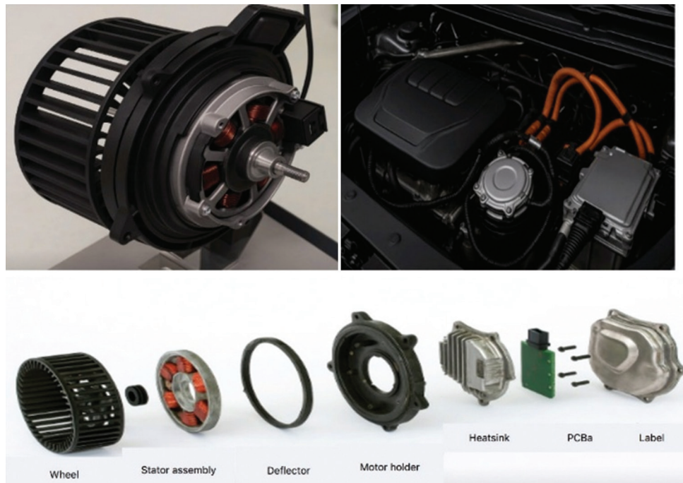
Fig. 2. A typical brushless direct current motor and its main components Abbreviation: PCBa: Printed circuit board assembly
