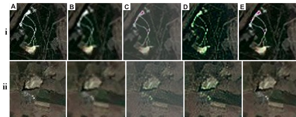
Fig. 2. Comparison of reconstructed details in distinct small targets (i and ii): (A) original image; (B) images reconstructed using VDSR; (C) images reconstructed using SRGAN; (D) images reconstructed using ESRGAN; and (E) images reconstructed using the proposed algorithm in this study Abbreviations: ESRGAN: Enhanced super-resolution generative adversarial network; SRGAN: Super-resolution generative adversarial network; VDSR: Very deep super-resolution
