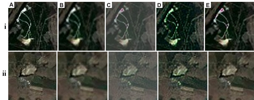
Fig. 2. Comparison of reconstructed details in distinct small targets (i and ii): (A) original image; (B) images reconstructed using VDSR; (C) images reconstructed using SRGAN; (D) images reconstructed using ESRGAN; and (E) images reconstructed using the proposed algorithm in this study Abbreviations: ESRGAN: Enhanced super-resolution generative adversarial network; SRGAN: Super-resolution generative adversarial network; VDSR: Very deep super-resolution
